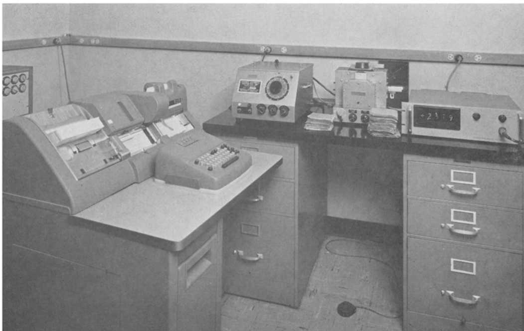
FIG. 2. Reflectometer, digital voltmeter and card punch assembly.
